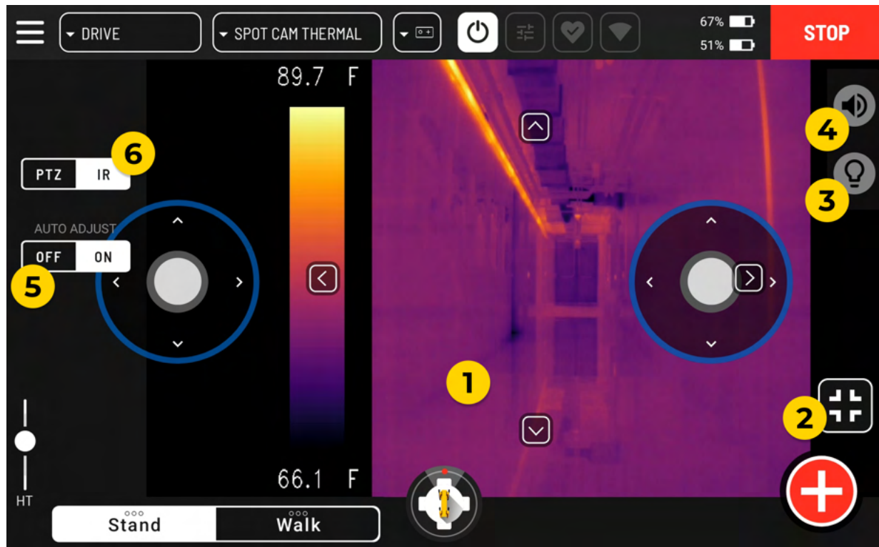
Thermal camera controls in the Spot App.
