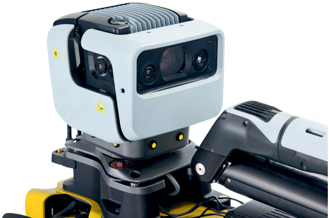
Spot Cam 2 mounted with a riser in the rear position.
