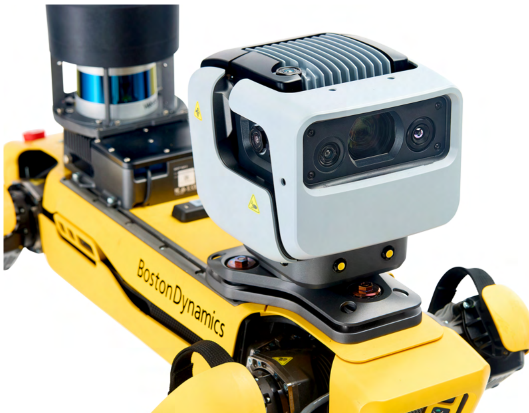
Spot Cam 2 mounted directly to the robot in the front position.
